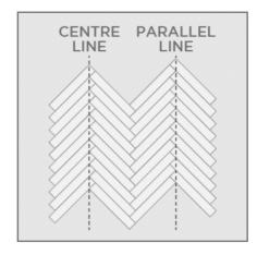
The apex of the herringbone pattern must be exactly in line with the guide string. Check the guide string regularly during installation
